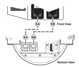
Figure 2-15 — Configuration of RJ-45 connectors
